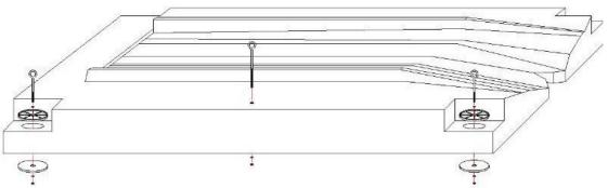
Install boat fender to floating dock and tighten rope from disks to eye screw on the floating dock. Frequent rope replacement may be needed from seasonal useage.
