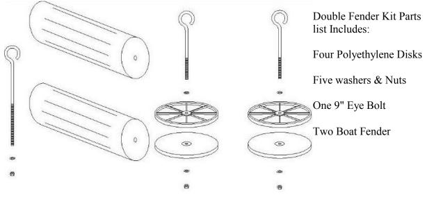
Place top disk over recess hole and run eye bolt through top disk hole through bottom disk hole. then use washers and lock nuts to tighten eye bolt & disk assembly.
