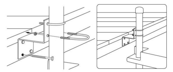
Recommended hardware: four 1/2 lag screws and four 1/2 washers that are Hot Dipped Galvanized
